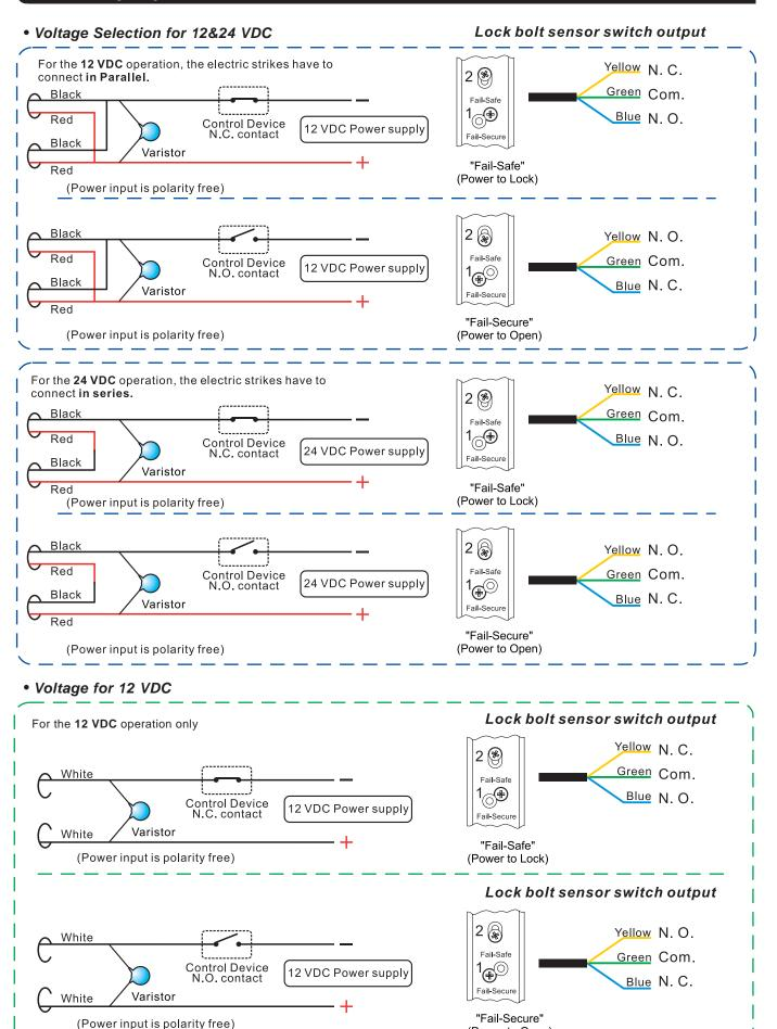
**NOTE:** The varistor (or diode) must be connected across the lock terminal (electromagnet...) operated by the device. The vartistor controls the overload produced by the strike coil (EMP).
